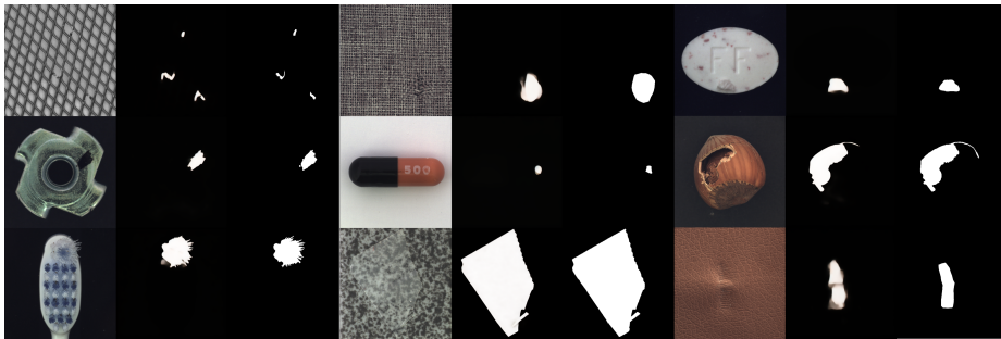
Fig. 17: Defect Detection Results. (Left: original image, Middle: prediction, Right: ground truth)
