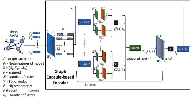
**Fig. 3:** The overall structure of the GCAPS network. Here,  $h$  is the embedding length, and bias terms are omitted for ease of representation.
