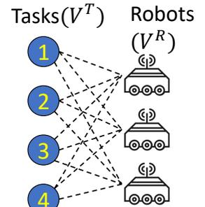
**Fig. 1:** Bigraph showing robot-task connections. The Bigraph weights is written as a matrix.
