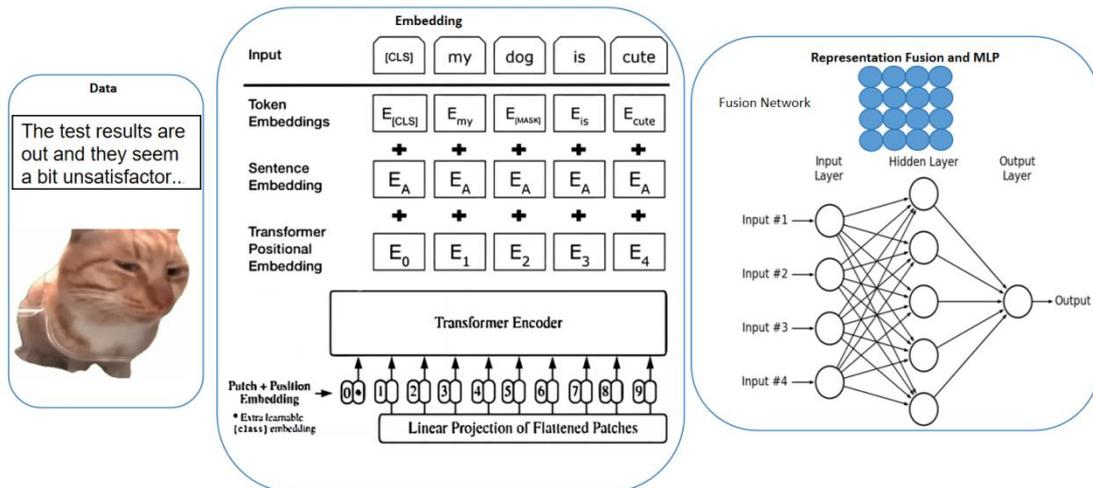
**Figure 4.** The fusion network based on transformer and tensor product
