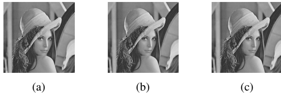
Figure 24: (a) Original image of 256 \times 256 pixels; Received images using (b) 16-QAM at SNR=10dB and (c) using 64-QAM at SNR=20dB.
