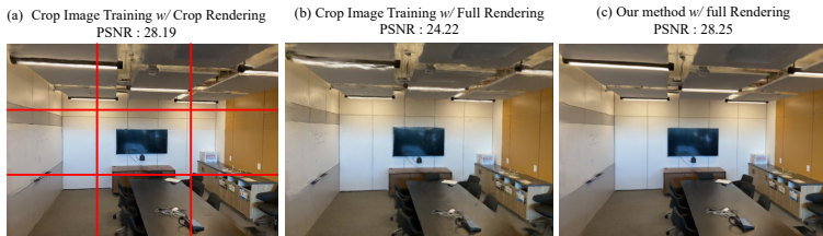
Fig. 8: Visualization of our method and crop image training. (a) Individual image patches are rendered separately and stitched together. (b) The entire image is rendered using the weights trained with our crop image training approach. (c) The entire image is rendered using our deferred back-propagation technique.
