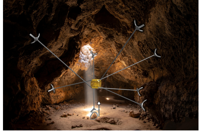
Fig. 1. ReachBot performs a sample-extraction manipulation task in a cave environment. By optimally planning (i) where to place the booms and (ii) the tensions in each boom, we ensure that this task is completed even with uncertain pose and wrench estimation, and stochastic failure modes.
