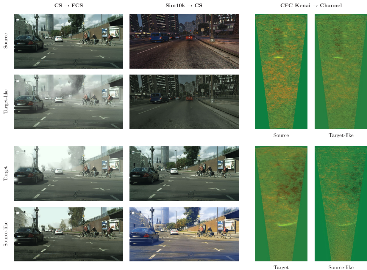
Figure 12: Exemplary results of our CycleGAN models. Source and target are the original images. Target-like and source-like are images translated by CycleGAN. Since FCS is derived from CS, CS \rightarrow FCS is the only case in which we have paired images and can therefore show the translation from source into target-like and from target into source-like for the same example.
