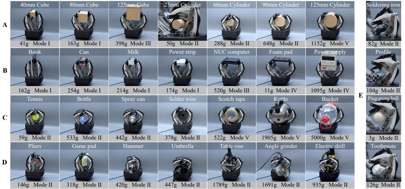
Fig. 11. Several demonstrations to verify the grasping performances in different Mode: grasp objects with regular shapes (A); grasp objects with regular planes (B); grasp objects with regular arc surfaces (C); grasp objects with irregular contours (D); grasp slender objects with one finger (E).
