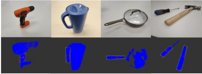
Fig. 4: Illustration showing PointGrasp output for 5 YCB objects with complex geometries. The top figure depicts the RGB image, and the bottom figure illustrates the handle identified and the grasping points (red) visualization of objects in the 3D box of the detected handles.
