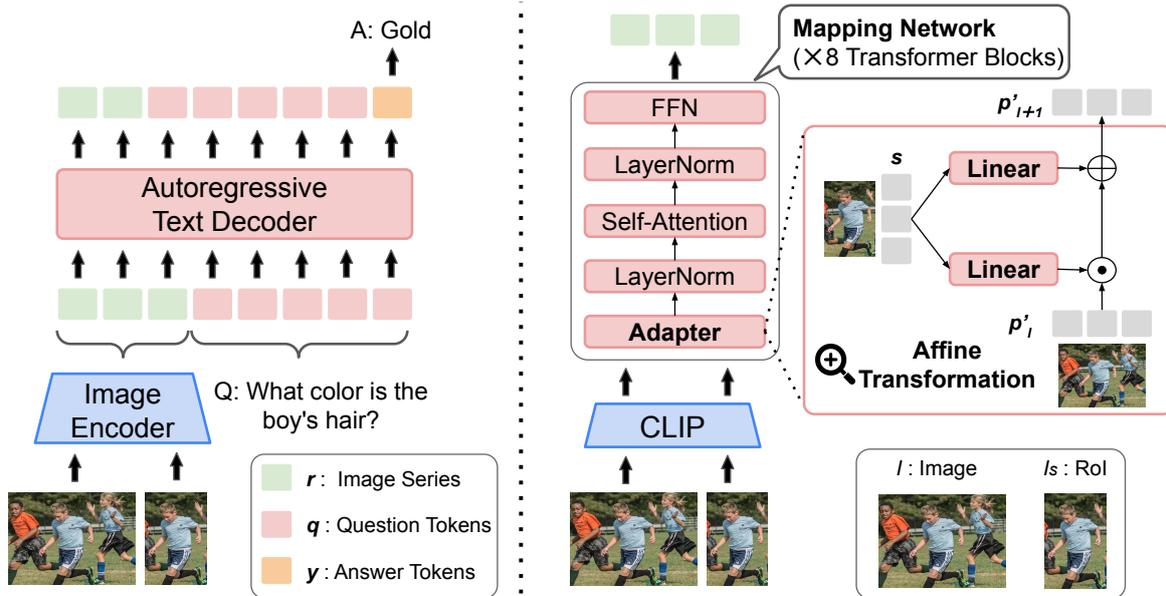
Figure 4: **Left:** Overview of proposed system **Right:** Details of Image Encoder architecture
