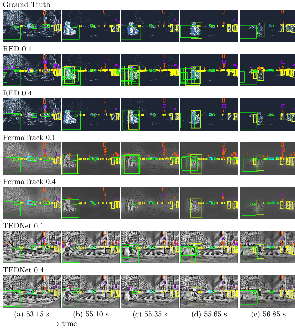
Fig. 6: A video sequence of the failure case with absolute timestamps, ground truth labels, and some detection results with different confidence thresholds. One car on the left remains still for a while, and one motorcyclist passes between the still car and the camera. The values after model names are the thresholds where the bounding boxes with confidence scores lower than those thresholds are filtered out. Bounding boxes with different colors correspond to different categories.
