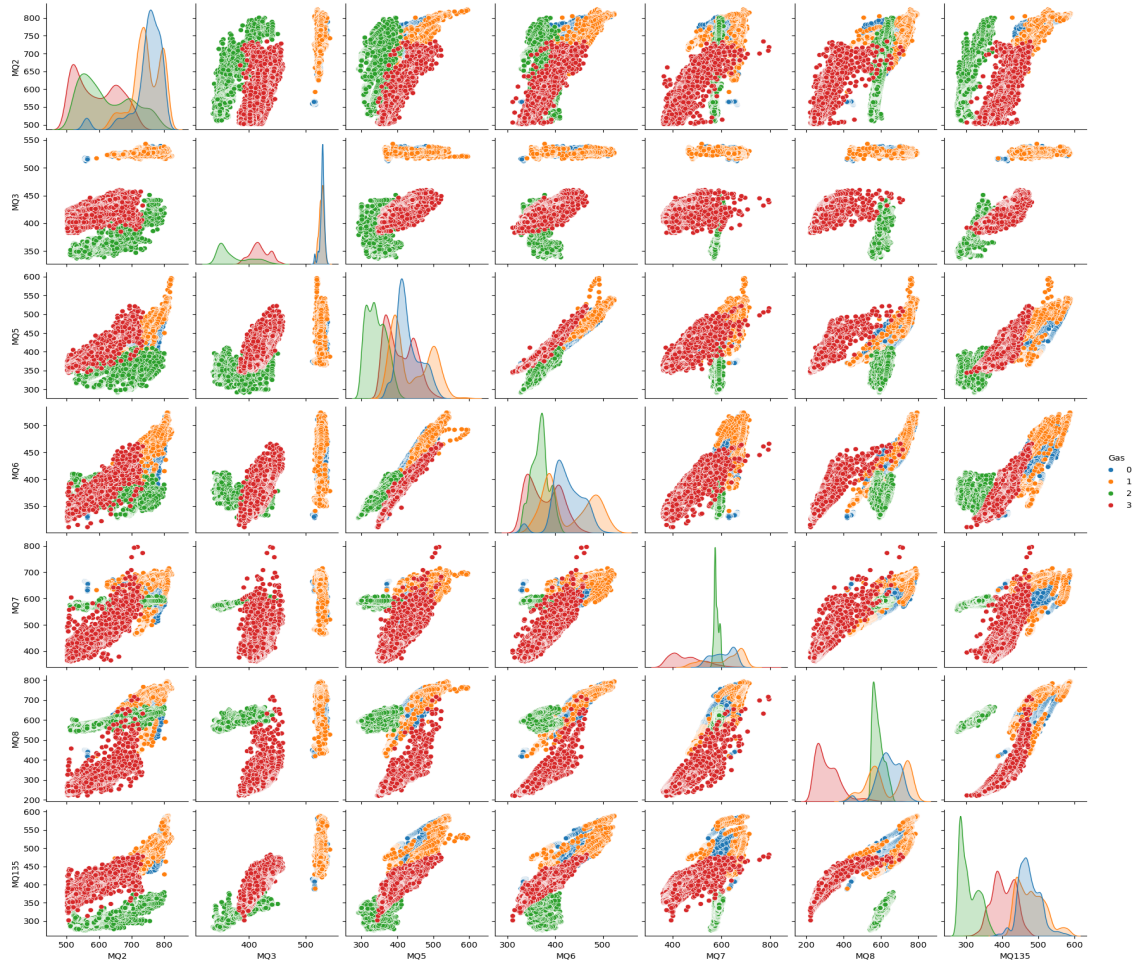
Fig. 7. Pair plot showing the relationships between sensors for different gas types.
