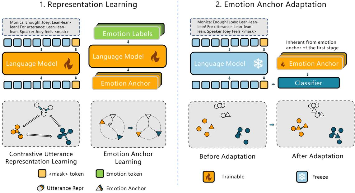
Figure 3: Overview of our proposed framework. **Left side** introduces representation learning, which is composed of utterance representation and emotion anchor learning. **Right side** describes the process of adapting emotion anchors to the optimal positions for classification.
