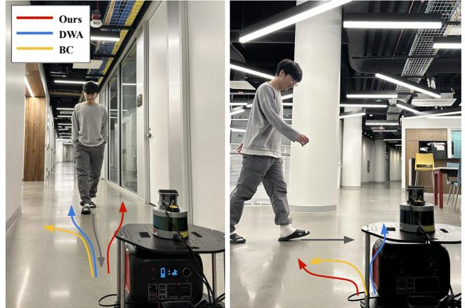
Fig. 1: The trajectories of our approach, VLM-Social-Nav (red), DWA (blue), and BC (yellow) approaches in the frontal encountering scenario (left) and the intersection scenario (right). The resulting trajectories show that VLM-Social-Nav demonstrates more social compliant behavior as it is instructed by a prompt (*i.e.*, Move to the right when passing by a person, and do not obstruct others’ paths).
