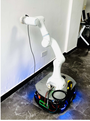
Fig. 6: Experiment setup. The end effector is equipped with a 6-axis force sensor and a cleaning tool, and the mobile manipulator is tasked to follow a motion/force trajectory along the rigid wall.
