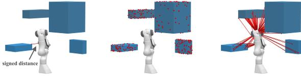
Fig. 2. Illustration of observations. Left: sCBF-INF takes the signed distance to the nearest obstacle as observation. Middle: For *fully-observable* environments, oCBF-INF uses a point cloud sampled uniformly on the obstacles as observation. Right: For *partially-observable* environments, oCBF-INF observes the point cloud from a mounted LiDAR sensor.
