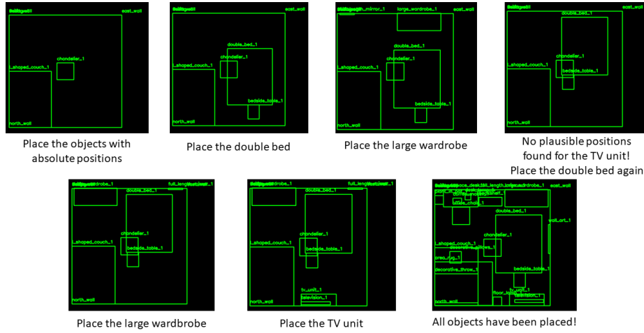
Fig. 3: Backtracking-based Scene Graph Layout. Starting from the scene graph specifying interior items as nodes connected with relative relationships, the backtracking algorithm solves for their absolute placement in the room. The algorithm reverses dead-end configurations and excels at object placement while respecting spatial constraints.
