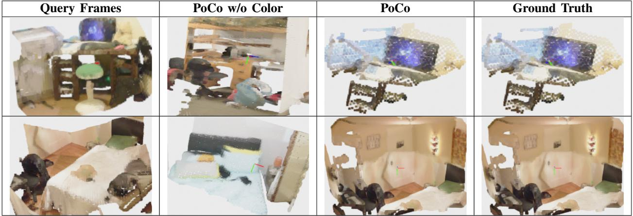
Fig. 8: **Benefits of Color Information.** The second and third columns show recall@1 frame from models w/o and with color information, respectively. After we remove the color information, the PoCo w/o Color model selects candidate frames only based on geometric information, where the desk (1st row) and the bed (2nd row) in matched candidate frames are structurally similar to the query frames, but their colors are very different.
