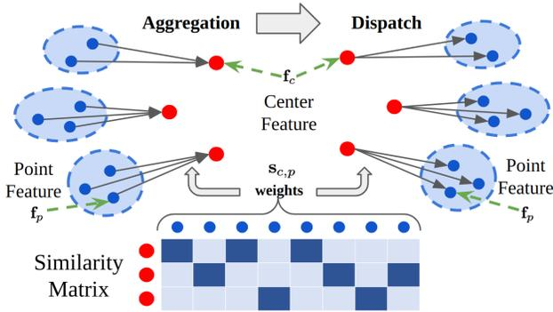
Fig. 4: **Cluster Block.** Red points are centers downsampled from the blue points. The blue points are grouped by the similarity of w.r.t. the red centers. Then the features of the blue points are aggregated to the centers by Eq. 3 and then the center features are dispatched to the points by Eq. 4.
