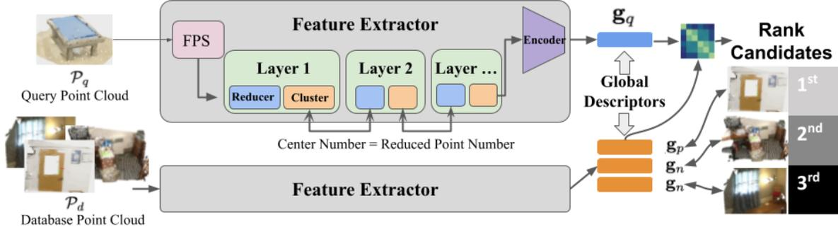
Fig. 2: **PoCo Architecture.** The input contains query and database frames and the model generates a global descriptor for each frame, and the descriptors are used to rank database frames by the similarities to the query frame. Note that the extractor consists of Farthest Point Sampling (FPS), an encoder, and layers of Reducers and Cluster blocks (see Fig. 3, 4).
