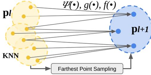
Fig. 3: **Reducer Block.** The blue circles are points in different levels. In Reducer Block, we use the Farthest Point Sampling method to downsample points  $\mathbf{P}^l$  to  $\mathbf{P}^{l+1}$  and aggregate the geometric and feature information of the  $K$ -nearest neighbors to the downsampled  $\mathbf{P}^{l+1}$  by Eq. 1.
