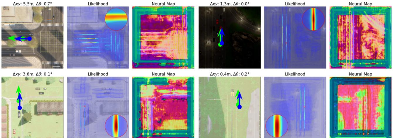
Fig. 4: **AGL-NET output visualization in CARLA simulation:** We use green arrow for the ground truth and blue arrow for the predicted pose. We highlight and enlarge the likelihood region near the ground truth in the read circle. Even in case of a larger location error (top left), the pose likelihood distribution have higher value along the lane of the road.
