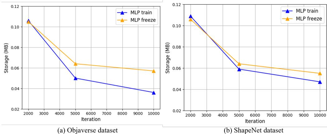
Figure 18: Triplane feature compression comparison. We used the ‘Car’ dataset for (b). We omitted the values before the 2000 iteration because the difference was almost negligible. The depicted storage sizes are only the compressed triplane feature sizes.
