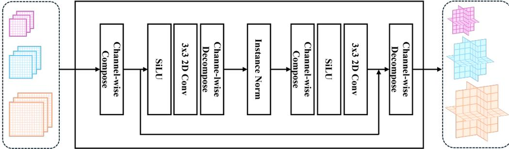
Figure 26: ResNet style 2D convolution block.
