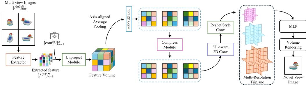
Figure 1: CodecNeRF encoder and decoder architecture. See (Section 3.1) for details
