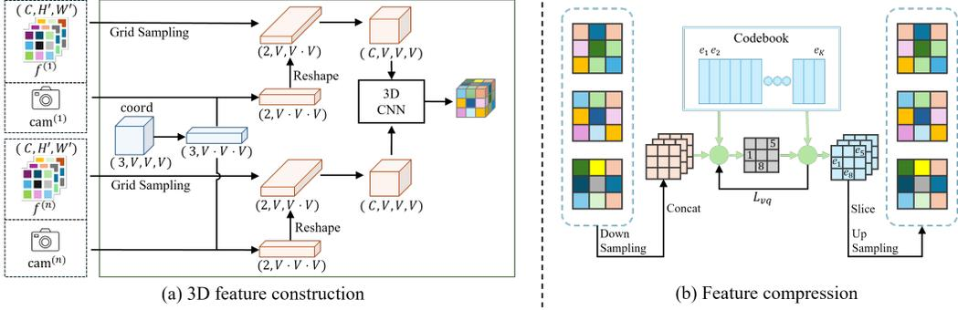
Figure 2: 3D feature construction and compression architecture. See (Section 3.2) and (Section 3.3) for details.
