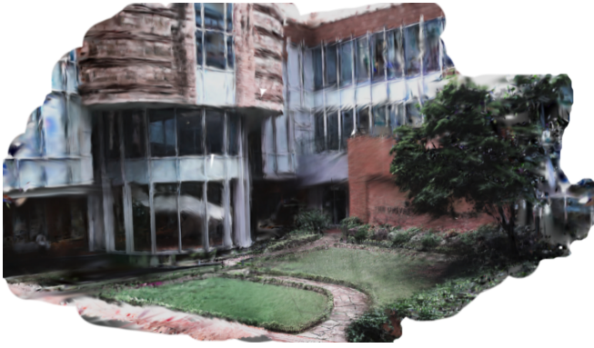
Fig. 3: The Gaussian map of the hku_campus_seq_00 sequence reconstructed by our Gaussian-LIC. The Gaussian map is visualized by SuperSplat 3 .
