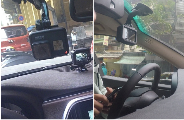
Figure 1. Positions of GoPro cameras used for data collection. A camera was attached to the windshield to capture a driver’s face and head movements. Another camera was placed on the dashboard, pointing out to the road.
