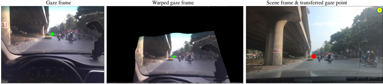
Figure 2. Matching result using RANSAC-Flow [37]. RANSAC-Flow is used to warp the gaze frame to the scene frame and transfer the gaze point (green dot) from the gaze frame to the scene frame (red dot). On an annotated dataset of 589 instances, the median and mean errors are 9.2 and 25.1 pixels, which are relatively small compared to the 1280 \times 720 size of the scene frame. The top right corner of the scene frame shows a circle with the radius of 25.1 pixels.
