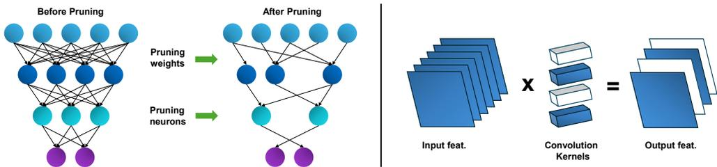
Fig. 4. Illustration of pruning methods: unstructured pruning (left), and structured pruning (right). Pruned components are shown in white color. Take note of the change in the pruned component's output dimensions.
