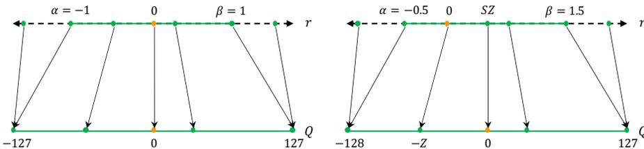
Fig. 5. Symmetric (left) and asymmetric (right) quantization representation [58]. Note that  $r$  represents the real value,  $S$  represents the real-valued scaling factor, and  $Z$  represents the integer zero point.
