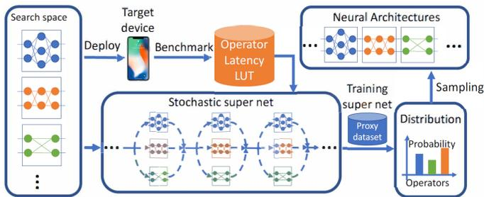
Fig. 8. The DNAS pipeline in FBNet [216].
