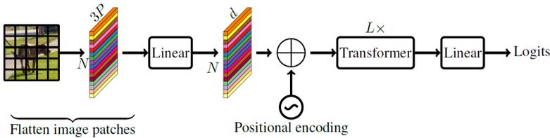
Fig. 3. Standard Vision Transformer, where  $P = h \times w$ ,  $h, w$  represents the height and the width of the images.  $N$  is the number of image patches,  $L$  is the number of transformer blocks, and  $d$  is the dimension [145].
