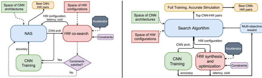
Fig. 11. Two different approaches for implementing NAS and hardware co-design [170].
