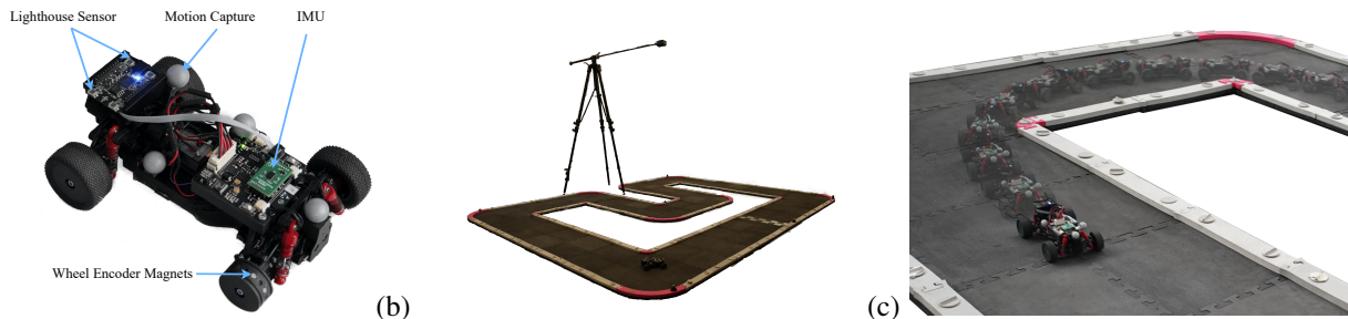
Fig. 1: (a) Chronos car based on a Kyosho AWD buggy model with custom electronics: IMU, wheel encoders with magnets in wheels, and Lighthouse positioning deck. (b) Track setup with Lighthouse base station. (c) Hardware experiment.
