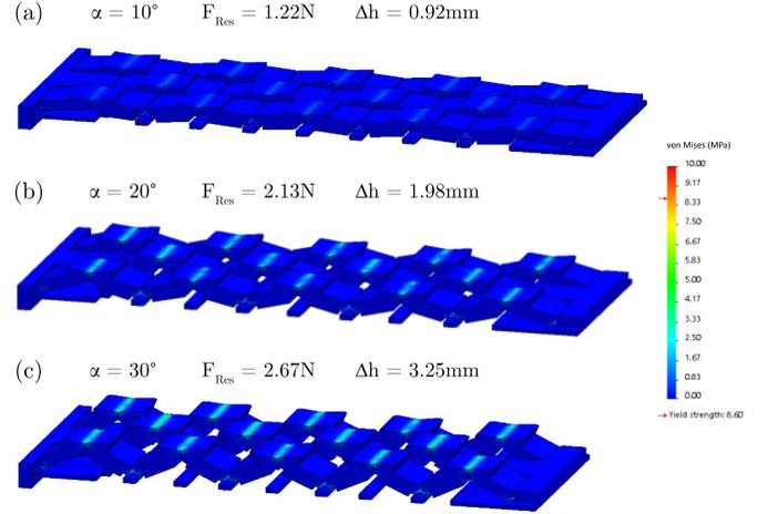
Fig. 4. Static simulation of the deformation required to fully fold each design with  $\alpha$  at values (a)  $10^\circ$ , (b)  $20^\circ$ , and (c)  $30^\circ$ . The resultant force (N) required to fully fold each specification is also shown. Simulation surface colours indicate the observed stress on the thermoplastic polyurethane (TPU) material.
