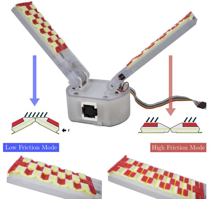
Fig. 1. Two-fingered two-degree-of-freedom gripper with fingers using the proposed origami-inspired variable friction (O-VF) surface. The controlled states of low friction (left finger) and high friction (right finger) are depicted, demonstrating the varying contact surfaces (black arrows).
