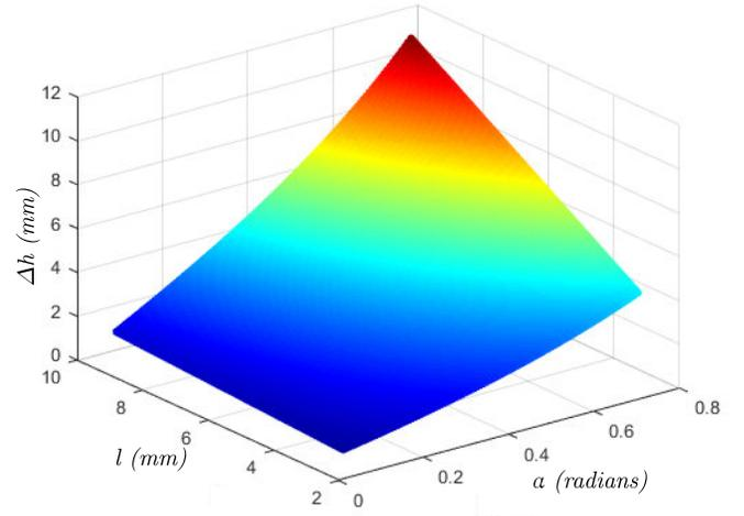
Fig. 3. Surface plot showing the relationship between the length of low friction area ( $l$ ), the folding angle ( $\alpha$ ), and change in thickness of the overall structure between friction modes ( $\Delta h$ ).
