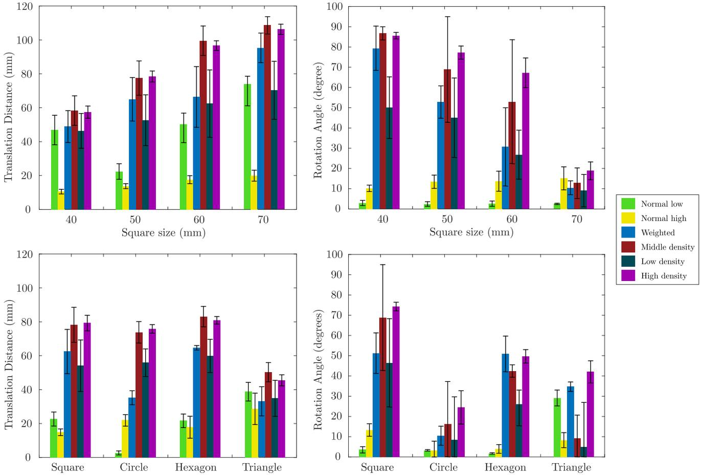
Fig. 11. Graphs showing the variation in translation and rotation capability for varying shapes and sizes for the six tested finger surfaces (low friction normal, high friction normal, weighted O-VF, medium density O-VF, low density O-VF, and high density O-VF), with standard deviation for each bar shown. Upper two graphs show the translational and rotational capability on 4 sizes of squares, while the lower two graphs show the same capability on 4 alternative shapes.
