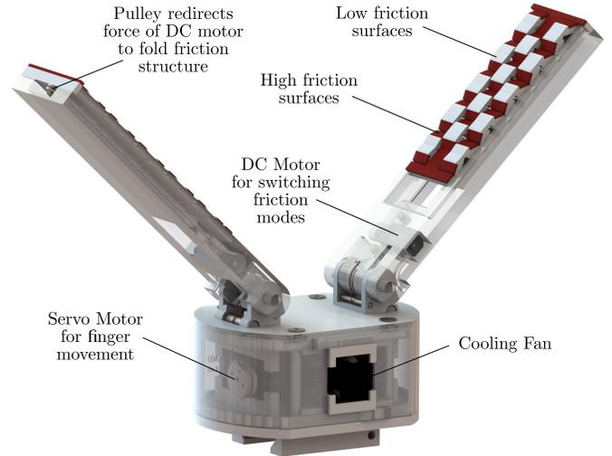
Fig. 6. CAD model profile of the developed gripper showing the visual and positional difference of the variable stiffness surfaces (left finger in high-friction mode, right finger in low-friction mode), as well as the positioning of the motors for finger motion and control of the friction.
