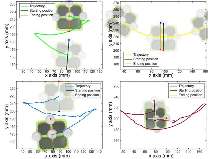
Fig. 10. Trajectories of a 40 mm square manipulated with normal and O-VF surface (medium density). **Top:** Low friction normal surface trajectory (left) and high friction normal surface trajectory (right). **Bottom:** Translational trajectory (left) and rotational trajectory (right) of O-VF surface. Red and blue dots indicate the two markers on the object. The green and yellow lines indicate the object starting and ending position, respectively.
