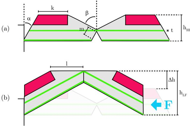
Fig. 2. Specifications of the folding pattern, defining the area ratio of variable friction surfaces and change in thickness between modes: (a) high friction and (b) low friction.
