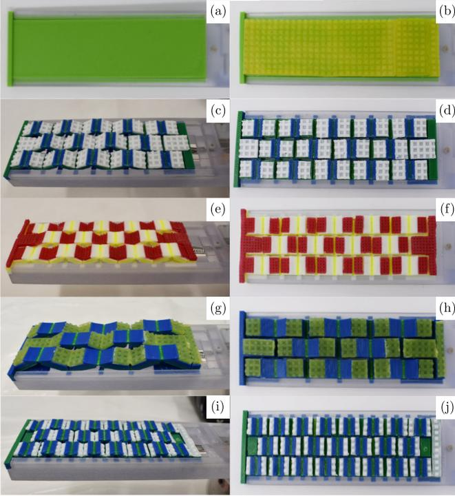
Fig. 7. Testing surfaces: (a) low friction normal surface, (b) high friction normal surface, (c, d) weighted O-VF surface, (e, f) O-VF surface with medium density, (g, h) O-VF surface with low density, and (i, j) O-VF surface with high density.
