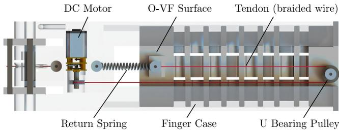
Fig. 5. Section view of the CAD model finger showing the actuation method and tendon routing on the rear of the O-VF surface.
