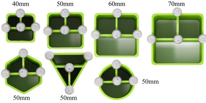
Fig. 9. The 7 different objects evaluated: 4 squares of width 40 mm to 70 mm and 3 alternative shapes of width 50 mm. The height of all the objects is 60 mm. Motion tracking marker positions for each shape are also shown.
