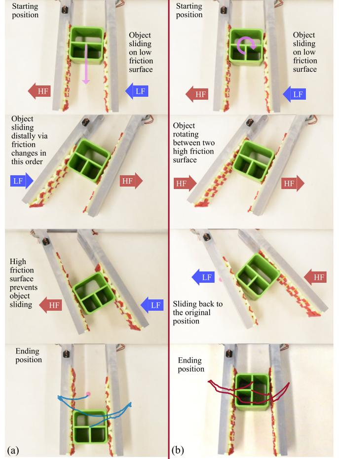
Fig. 8. Method for achieving translation (a) and rotation (b) of a 50 mm square object by actively controlling the variable friction surfaces while actuating the fingers. HF indicates high friction surface activated. LF indicates low friction surface activated. The arrow represents the finger moving direction. The blue and red curves in the final row show the trajectories of the manipulated objects. Further object manipulations can be seen in the accompanying video.
