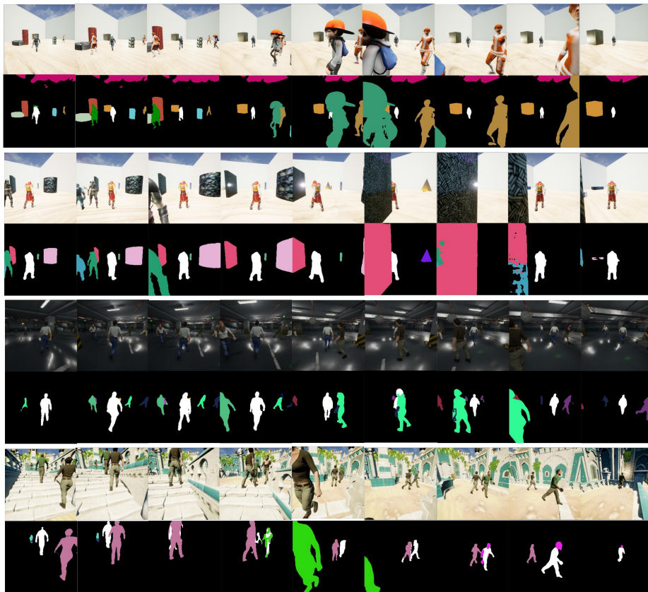
Fig. 7: The tracking demonstration of our agent in Virtual environments. The color image is the first-person view observation of the embodied agent. The mask on the bottom of the color image is the corresponding text-conditioned segmentation mask based on DEVA.
