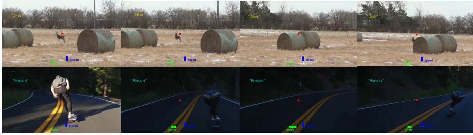
Fig. 4: The output actions of our agent in two video sequences from VOT Challenge [20]. We separately use “Deer” and “Person” as prompts. The central red point signifies the image’s center. The bottom green rectangle’s width indicates angular velocity control from -30^\circ/\text{s} to 30^\circ/\text{s} , while the bottom blue rectangle’s height indicates linear velocity control from -1 \text{ m/s} to 1 \text{ m/s} .
