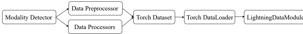
Figure 2: Interdependency among data modules: Each module from left to right serves as a prerequisite for the subsequent one.
