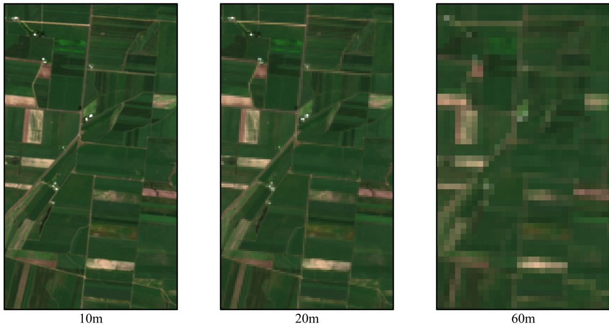
Figure 5: Spatial resolution comparison of available Sentinel-2 resolutions. Sentinel-2 offers four bands at 10m resolution, ten bands at 20m resolution and twelve bands at 60m resolution
