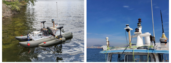
Fig. 2: Data collection platform ( left ): our custom ASV Catabot , ( right ): human-driven ship equipped with sensors.
