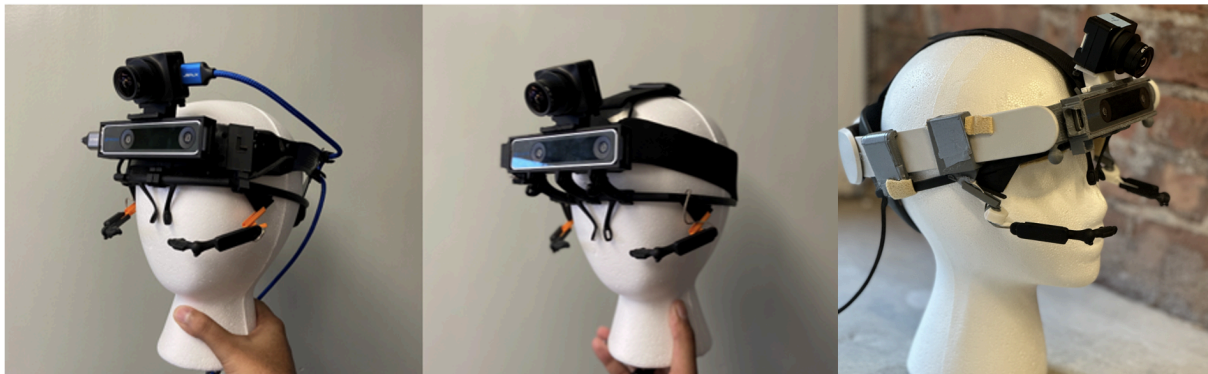
Figure 3: (Left) hard plastic mount; (Middle) elastic strap mount; (right) Virtual reality headset mount. The right mount also shows the custom ball joint eye extenders.
