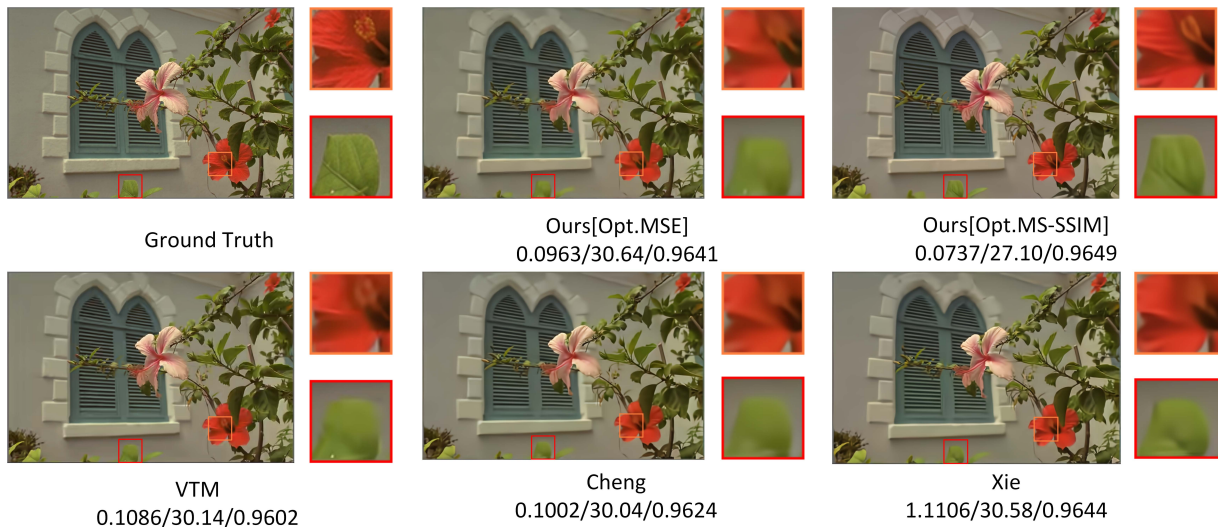
Fig. 8: Visual comparisons of decompressed image of “kodim07.png” from Kodak dataset based on different methods. The subfigure is titled as “bitrate/PSNR/MS-SSIM”.
