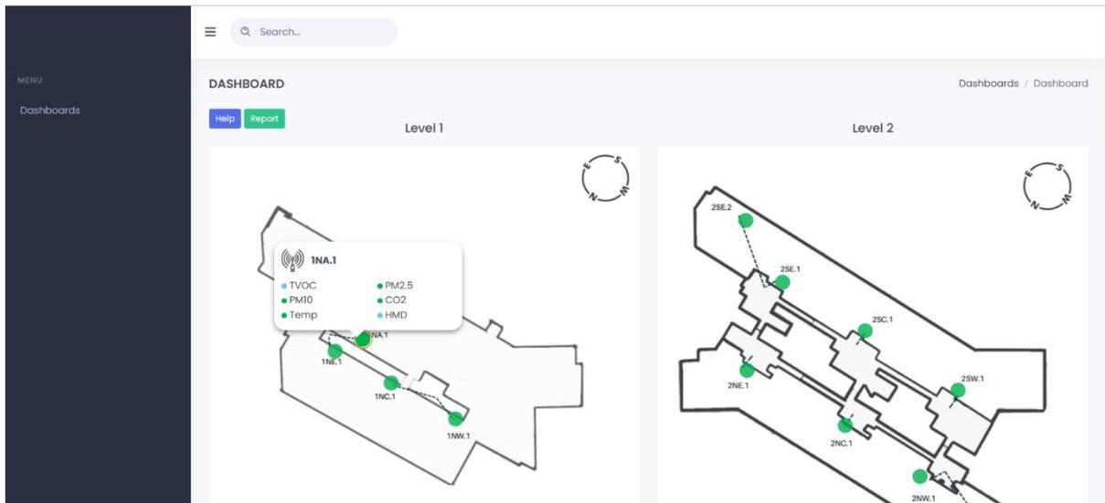
Figure 3. The developed air quality monitoring dashboard for a multi-tier building.
