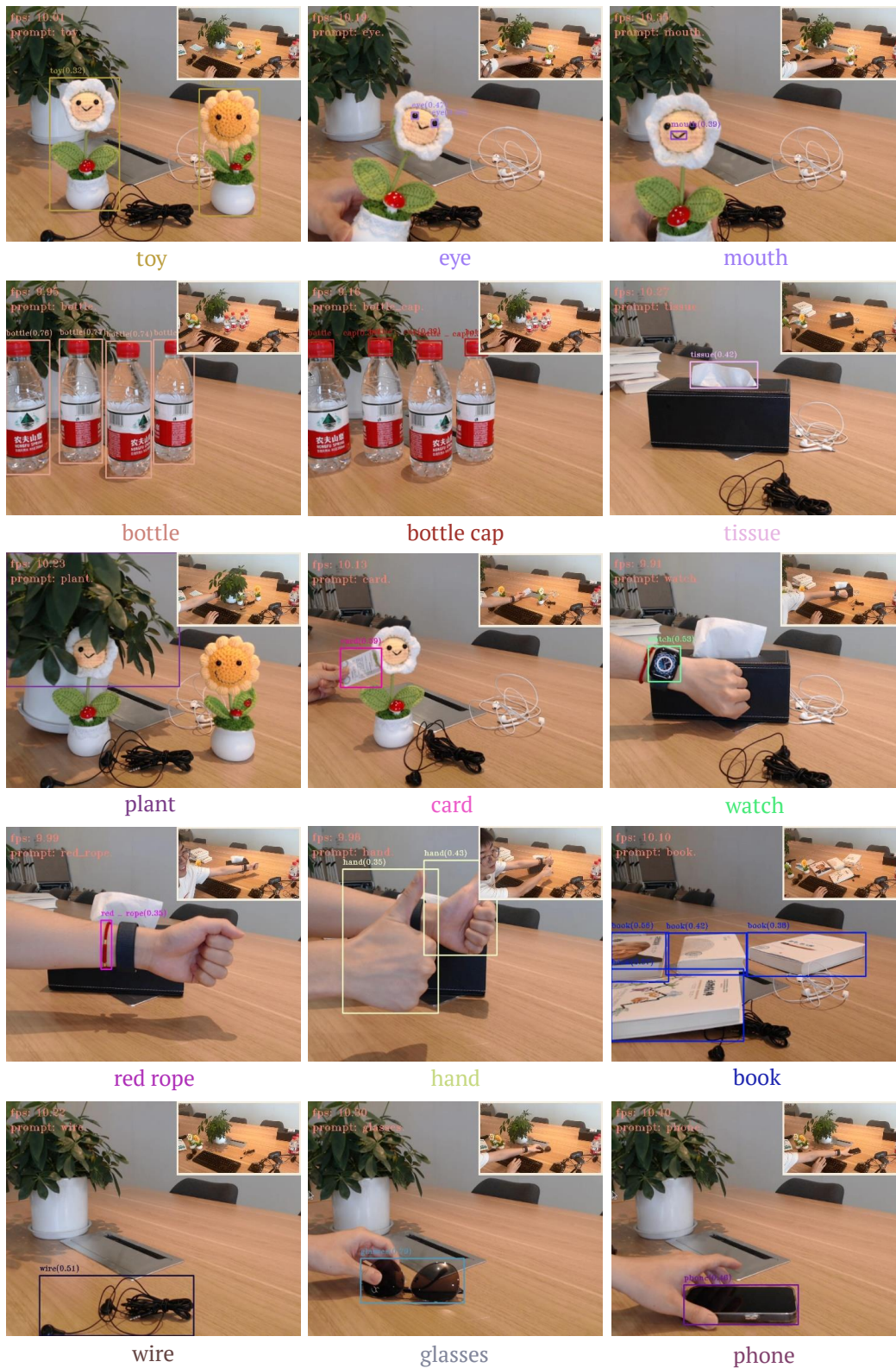
Figure 16: The visualization of Grounding DINO 1.5 Edge on NVIDIA Orin NX. The top left of the screen displays the FPS and prompts, while the top right shows a camera view of the recorded scene.
