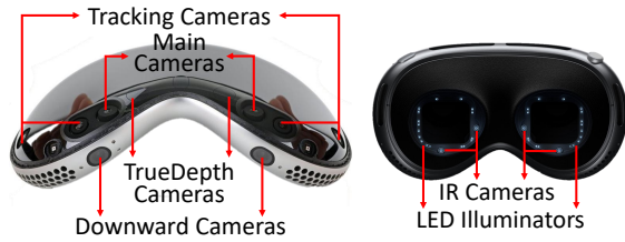
Figure 2: Cameras on Vision Pro.
