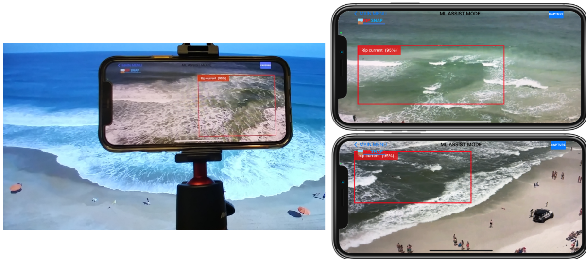
Figure 5: Appearance of the RipSnap app with examples of rip currents detected by the app. The location of the rip current is visualized using the red bounding box with the label and the confidence score of detection.
