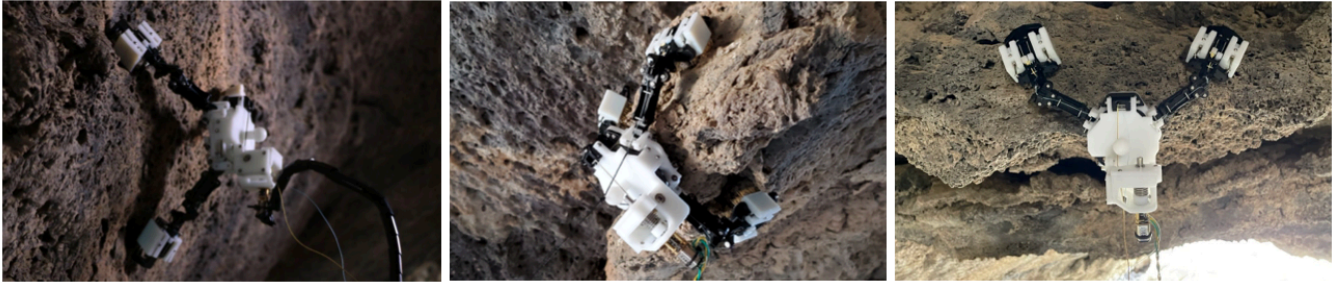
Fig. 4. In the field test, the microspine gripper was capable of grasping a variety of different rock surfaces, ranging from hemispherical (left) to ledge-like features (middle, right). These results provide confidence that the microspine gripper will successfully grasp highly irregular lavic rock surfaces.
