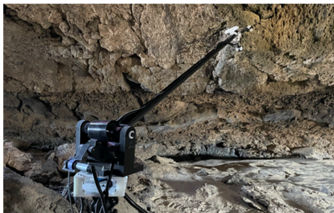
Fig. 1. ReachBot is a robotic concept that uses extending booms as prismatic limbs to navigate difficult terrain. Shown in a rendering (top) is the full ReachBot configuration overlaid on a photograph of the field test site in the Lavic Lake volcanic field in the Mojave Desert. During this field trial, a single-boom prototype (bottom) was tested to demonstrate a boom deployer, perception system, and microspine gripper.
