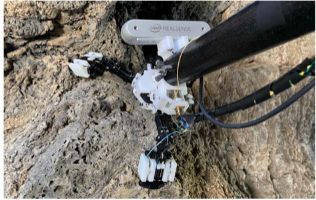
Fig. 2. A custom microspine gripper was developed and field tested. Shown is a CAD rendering (top) of the microspine gripper. Also shown is a photograph (bottom) from the field test of the gripper successfully grasping a rock while mounted at the end of an extended boom.
