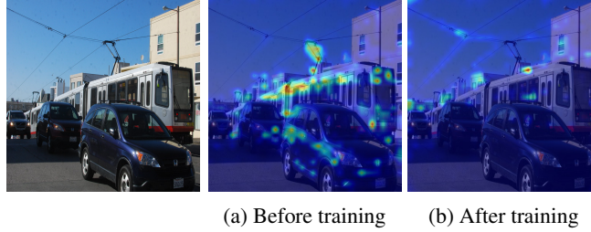
Figure 4: Attention map visualization: pre-trained DINOv2 focuses on irrelevant foreground objects e.g. vehicles. Whereas attentions of EفوVPR after training are shifted to scene layout and building structures such as cables and windows.
