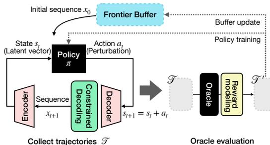
Figure 1. **Overview of LatProtRL.** At each round, an RL policy  $\pi$  acts to collect trajectories  $\mathcal{T}$  for a fixed number of episodes. After  $\mathcal{T}$  are collected, the reward is calculated based on the feedback from an oracle. The trajectories with calculated rewards,  $\mathcal{T}'$ , are used to train the policy using an on-policy RL algorithm.
