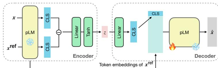
Figure 2. **Variant Encoder-Decoder Architecture.** Given an input sequence, the encoder calculates a representation that is used by the decoder to reconstruct the original sequence. The term CLS represents the embeddings for the classification token in ESM-2.
