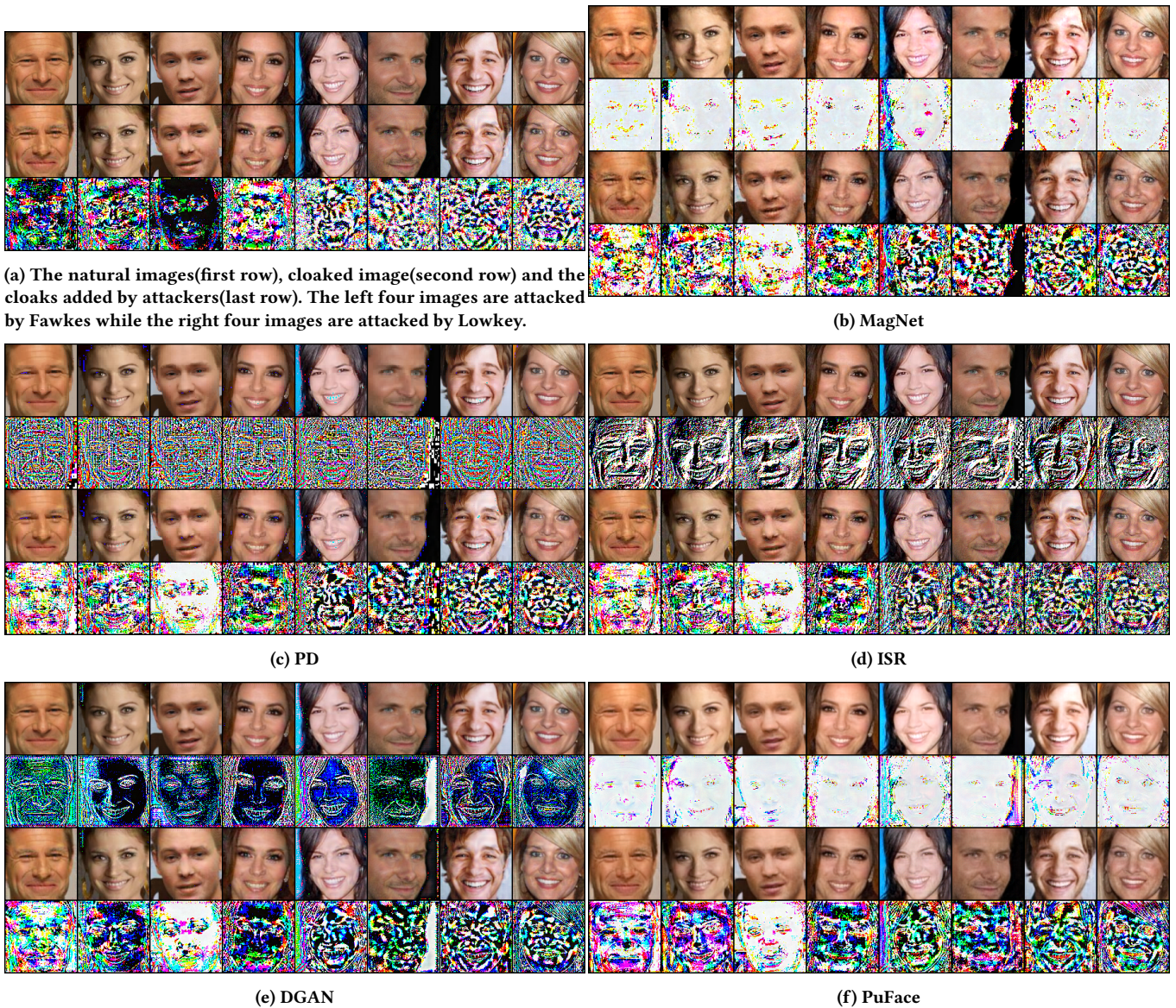
Figure 3: The reconstructed results of different defenses. Figure 3a shows the natural images, cloaked images and the cloaks between them. Following are 5 visual comparison of different defenses. In each figure, the first and third row present the reconstructed images of natural and cloaked images respectively, and the second and last row show the difference between them and the natural images.
