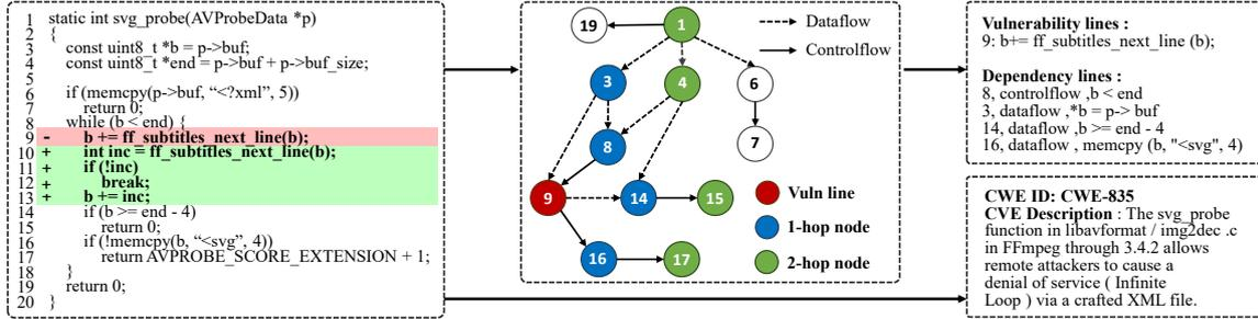
Figure 2: An example of vulnerability feature extraction
