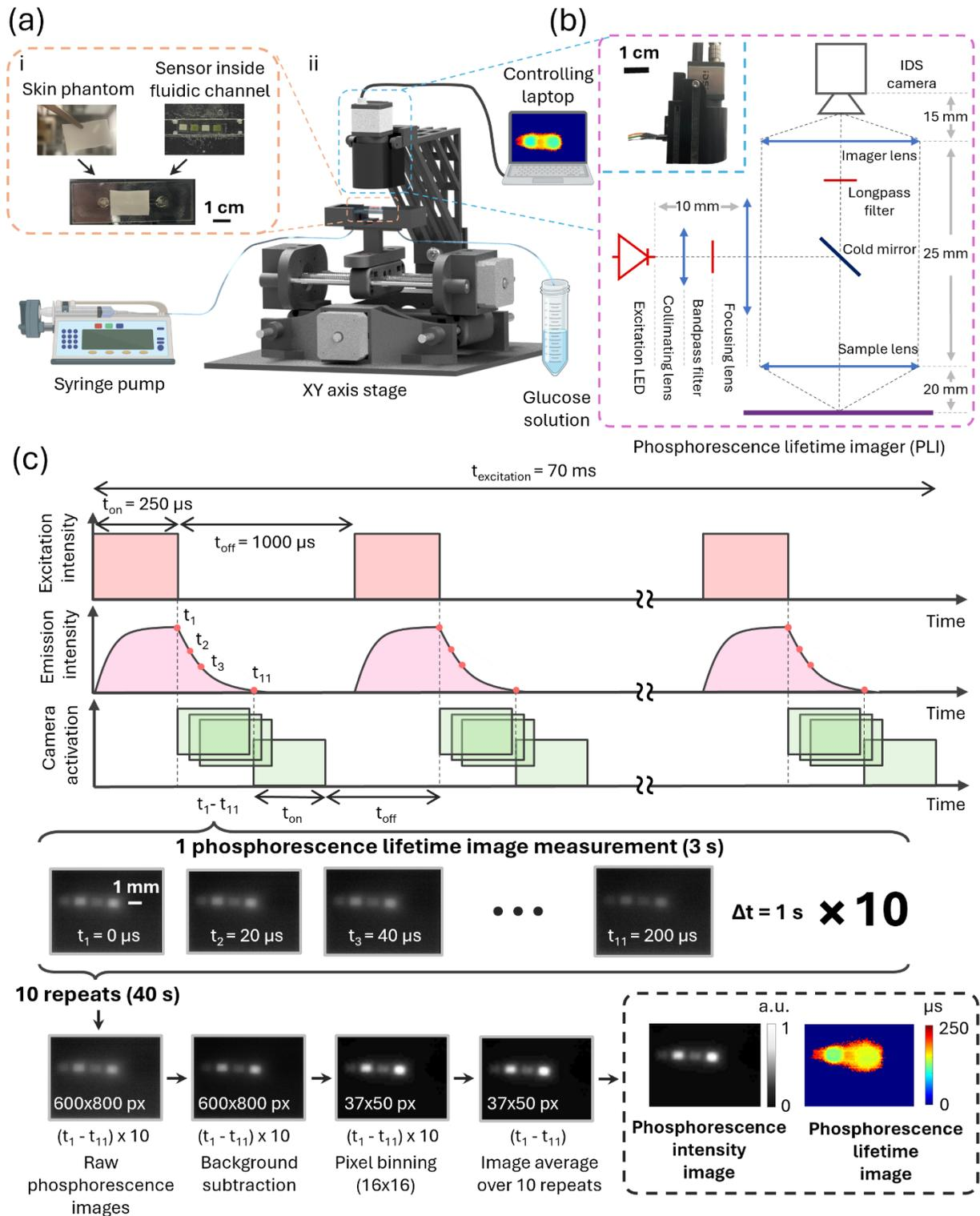
**Figure 2.** (a) Experimental setup for *in vitro* testing of the PLI reader; (b) PLI reader structure; (c) Reconstruction of the phosphorescence intensity and phosphorescence lifetime images.
