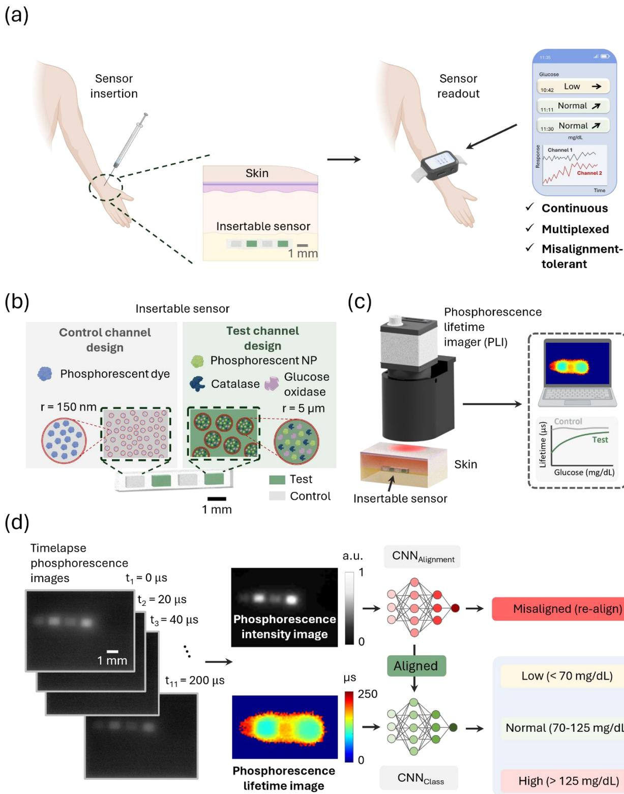
**Figure 1.** (a) Overview of optical continuous glucose monitoring, featuring an insertable/implantable passive biosensor and a wearable reader; (b) Insettable sensor structure; (c) Operation of the phosphorescence lifetime imager (PLI); (d) Neural network-based processing of phosphorescence images for misalignment-resilient classification of glucose concentration levels (low/normal/high).
