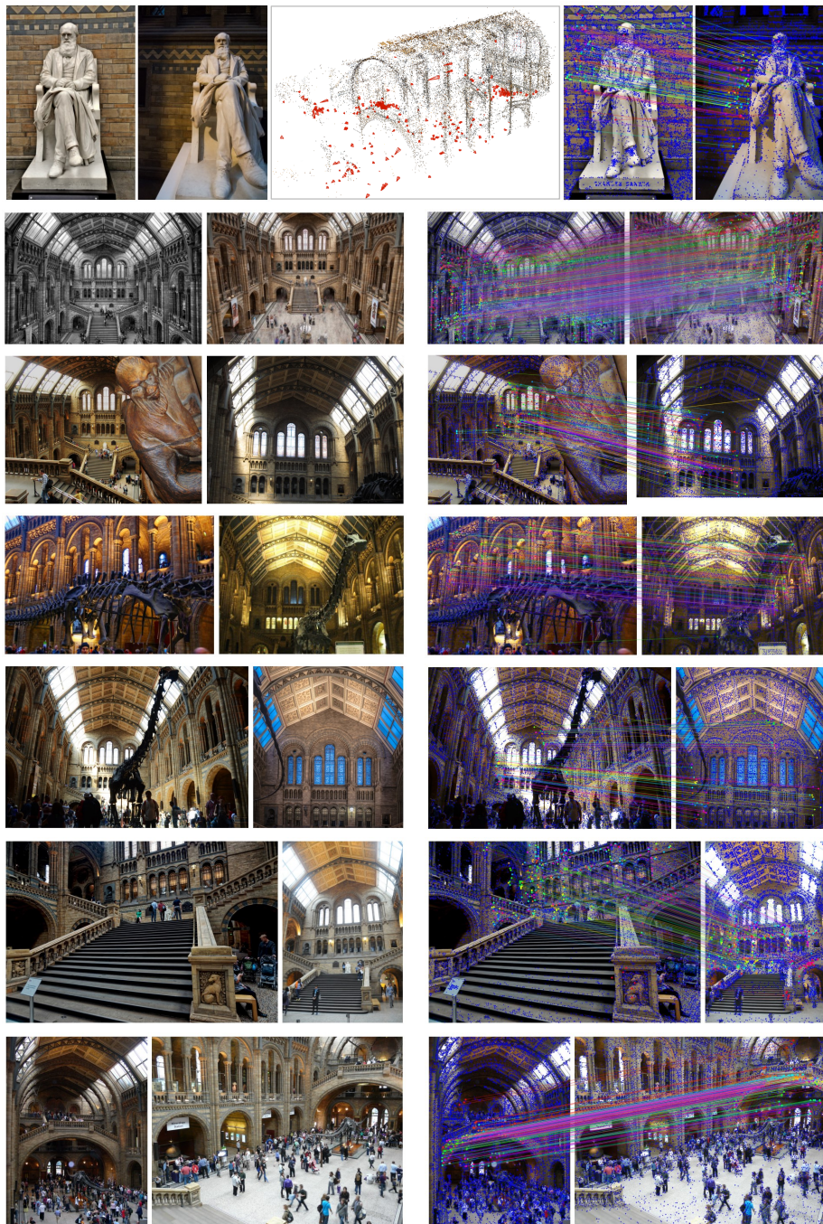
Fig. 9: Feature matching visualization of the Natural History Museum’s interior in London, with the SfM reconstruction shown in the middle of the top row. On the left, selected image pairs are shown, and on the right, the extracted keypoints (in blue) and their matches (in color-coded) from the two-view geometry table in COLMAP [44] database are displayed.
