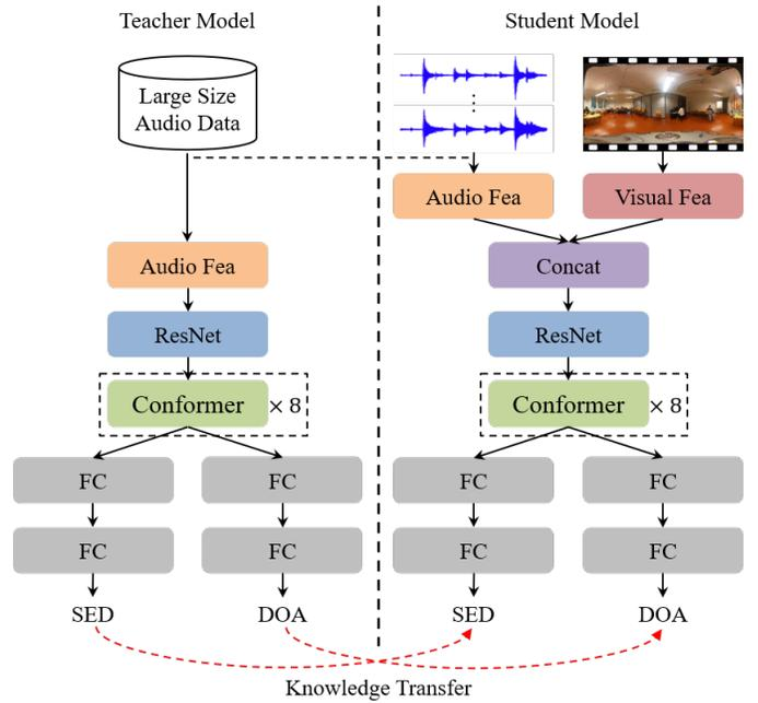
Fig. 1. The proposed AV-SELD model is based on cross-modal teacher-student learning and multi-modal fusion, as shown in the overall architecture.
