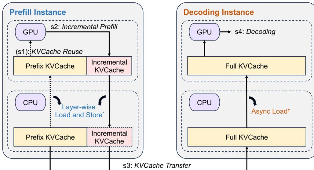
Figure 4: Workflow of inference instances. (\*) For prefill instances, the load and store operations of the KVCache layer are performed layer-by-layer and in parallel with the prefill computation to mitigate transmission overhead (see §5.2). (†) For decoding instances, asynchronous loading is performed concurrently with GPU decoding to prevent GPU idle time.
