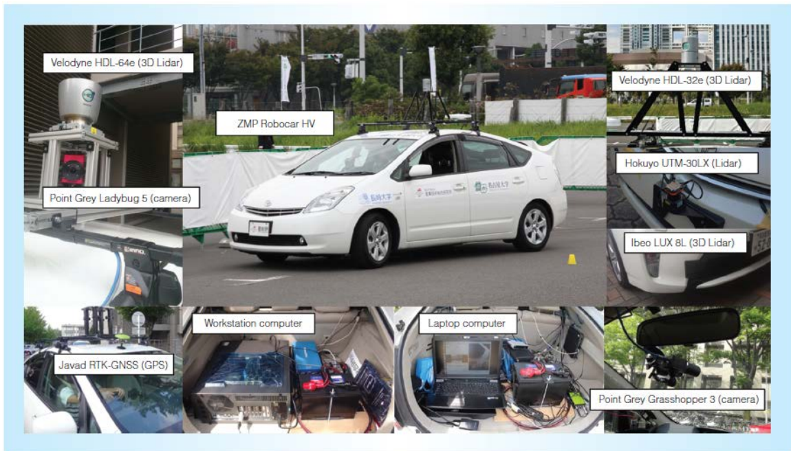
Figure 2 Example of hardware configuration of autonomous vehicle [1]
