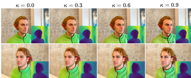
Fig. 5. Qualitative results under different hyper-parameter settings. Rendered RGB and depth representations illustrating the implications of different DDCM coefficient \kappa on 3DGS editing.
