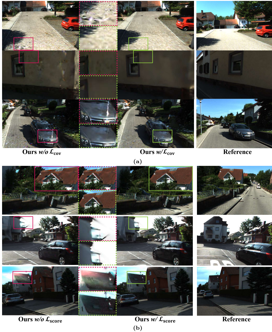
Fig. 6: Qualitative ablation results on (a) \mathcal{L}_{cov} and (b) \mathcal{L}_{score} on EVS. \mathcal{L}_{cov} effectively guides the Gaussian covariances to faithfully cover the scene surface, yielding noticeably less cavity and better geometry. \mathcal{L}_{score} effectively improves broken textures, geometry, and removes floating artifacts.
