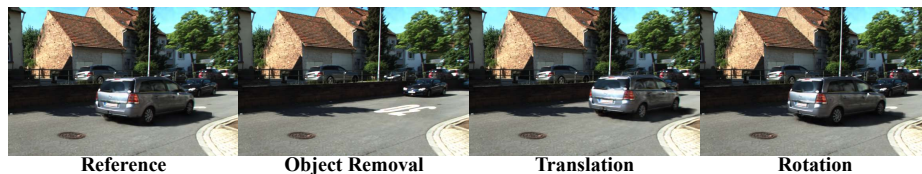
Fig. 7: Scene editing results. Since our method models dynamic objects on its own canonical space separated from world coordinate, the reconstructed object can be re-located or removed by manual adjustments.
