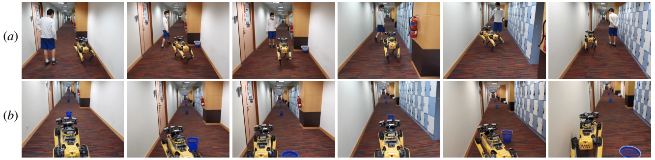
Figure 11. Illustrations of challenging real-world scenarios. (a) Task i.: The robot avoids the adversary by predicting its movement. (b) Task ii.: The robot successfully bypasses the basket that is not in the robot camera view.
