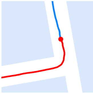
Figure 3. An illustrative representation of the Local Path and Environment (LPE) intention. It is a cropped section of the map, where the robot’s historical path is visualized as a continuous red curve, while the planned future trajectory is delineated by a distinct blue curve.
