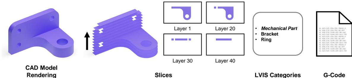
**Figure 2:** Different data formats in Slice-100K. We build our dataset using CAD models (STL files) and their renderings. Furthermore, we slice these STL files to generate G-code (build direction shown by black arrow) and their categorical classifications.
