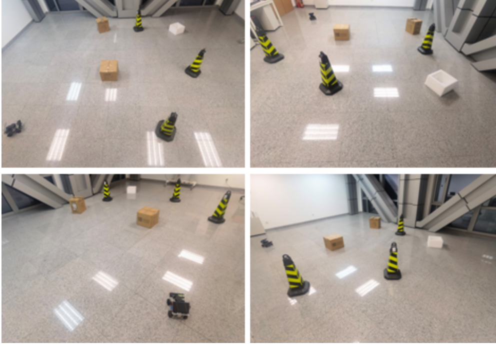
Figure 7: Real-world experimental setups designed to test the obstacle avoidance capabilities of autonomous systems. The images depict various configurations of obstacles, such as cones and boxes, arranged in a controlled indoor environment to simulate different urban and semi-urban scenarios. These setups assess the robustness and adaptability of navigation algorithms in dynamically changing and physically constrained spaces.
